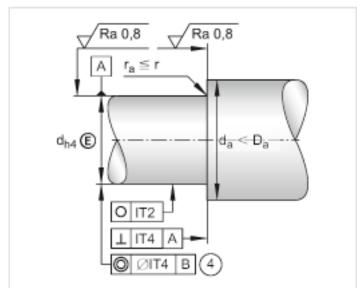
Design of housing and shaft (threaded spindle)
