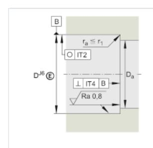
Design of housing and shaft (threaded spindle)
