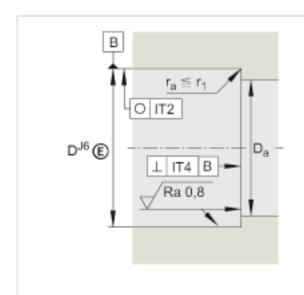
Design of housing and shaft (threaded spindle)
