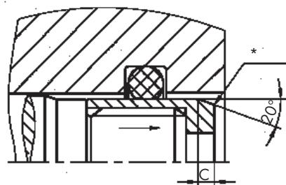
■ Tips of screws and installation housings for other sealing and guiding elements should be covered by an assembly sleeve.
