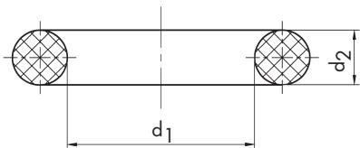
The O-ring designation is given from the dimension of its inner diameter and the cross section thickness in mm, the name of the material and its hardness (elasticity)
