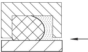
When ready to operate, the medium pressure promotes the deformation and increases the sealing effectivity. If the pressure drops to "zero", the deformation reverts almost to the fitted state.
